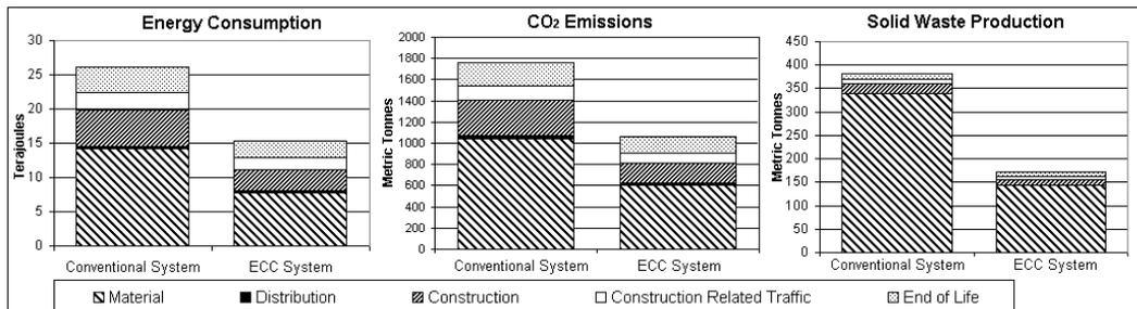
**Figure 2: Preliminary Life Cycle Inventory Results for the Conventional Concrete System and the ECC System over a 60-year time horizon.**
