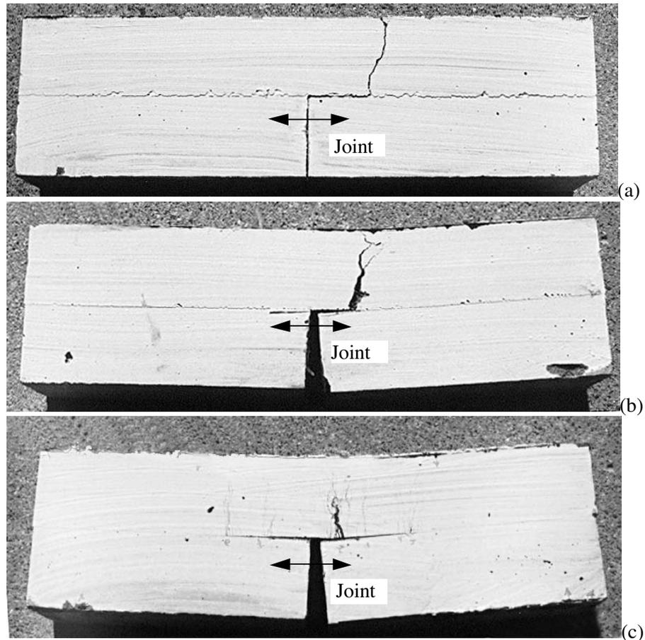
**Figure 4:** Failure modes of (a) PC/PC, (b) SFRC/PC and (c) PE-ECC/PC overlay systems.
