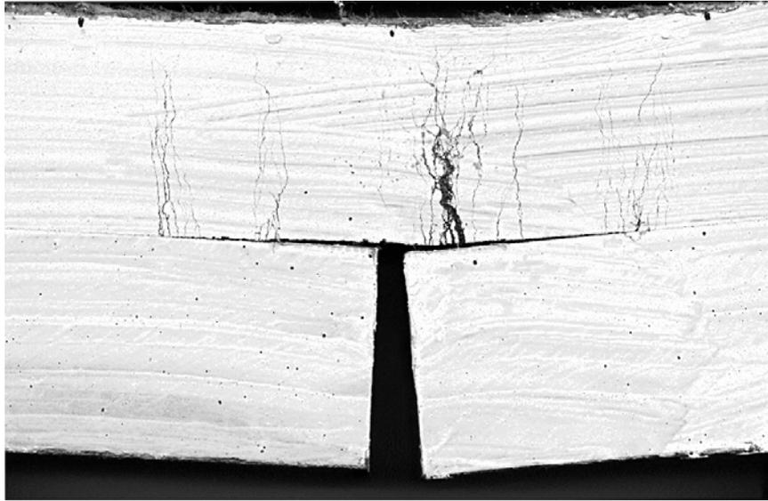
**Figure 6:** Close-up view of the kink-trap mechanism in the PE-ECC/PC overlay system.
