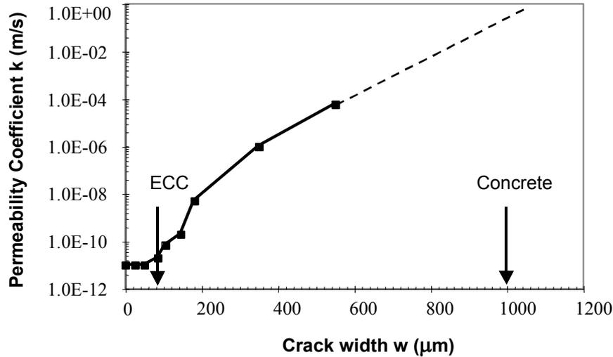
**Figure 11:** Experimentally measured permeability coefficient as a function of crack width in plain concrete (adapted from [11]). The dashed part of the curve is extrapolated from the experimental data (solid curve).
