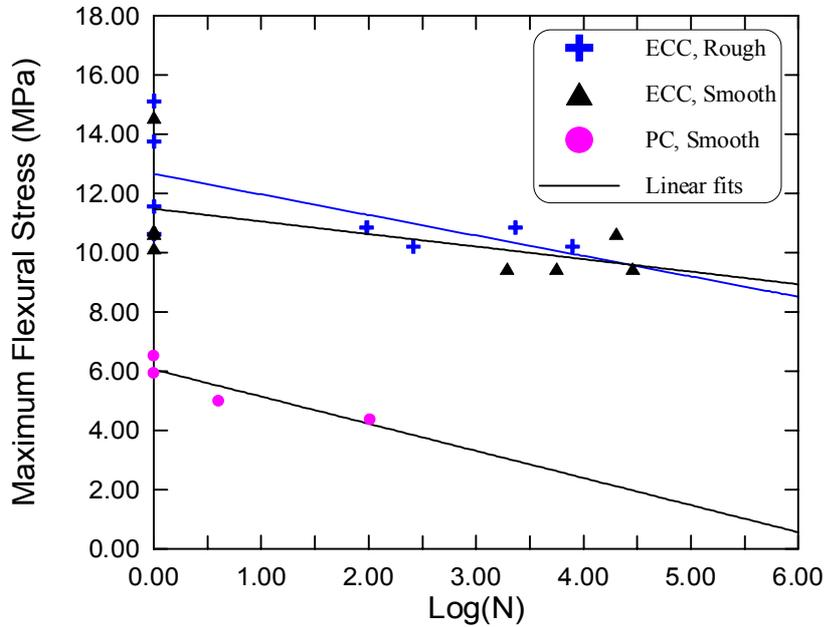
**Figure 8:** S-N curves of PVA-ECC/PC and PC/PC overlay systems tested under flexural fatigue loading.
