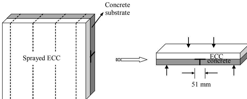
Figure 9: Spray PVA-ECC/PC overlay specimen.
