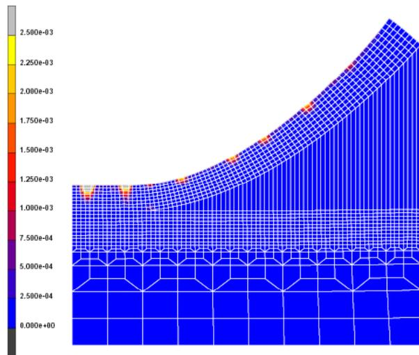
**Figure 13 b):** Contour bands of normal cracking strain (%) on deformed mesh (magnification 100x) for SFRC overlay at 10 days
