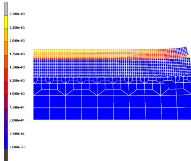
**Figure 13 c):** Contour bands of normal cracking strain (%) on deformed mesh (magnification 100x) for ECC overlay at 100 days (adapted from [7]).
