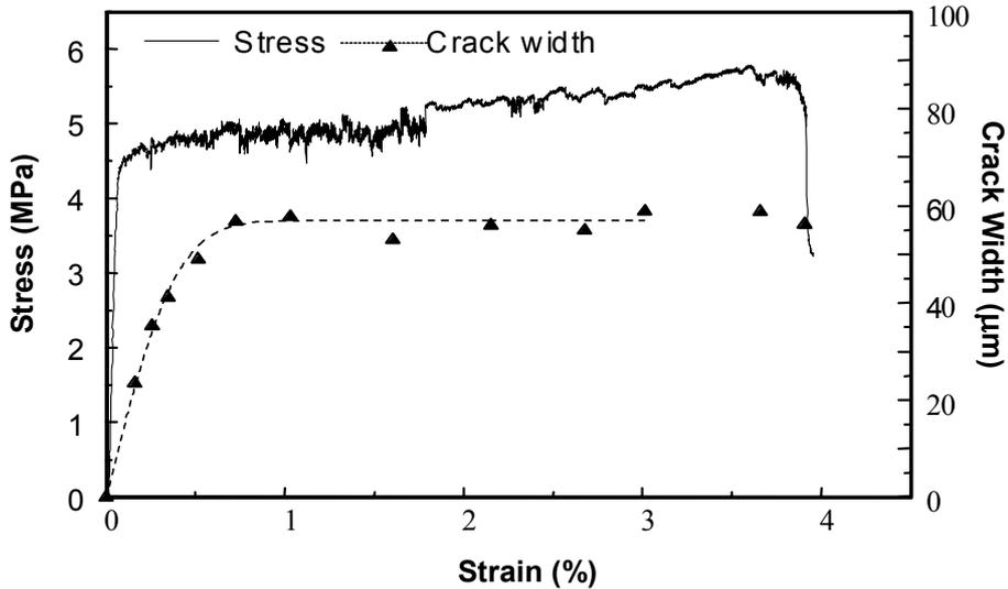
**Figure 1:** A typical stress-strain curve of ECC, showing high tensile strain capacity, and tight crack width control.
