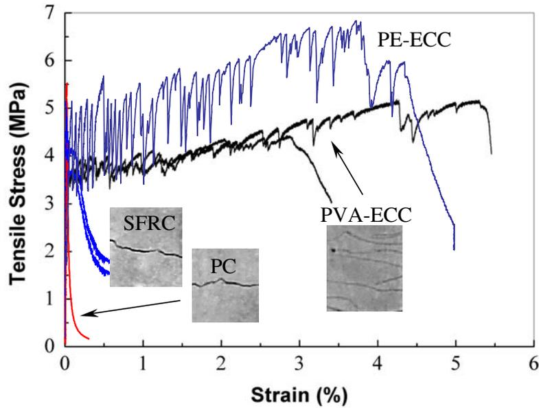
**Figure 3:** Tensile stress-strain curves of PC, SFRC, PVA-ECC and PE-ECC.
