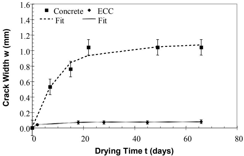
**Figure 12:** Crack width development for PVA-ECC and normal concrete in restrained drying shrinkage test.
