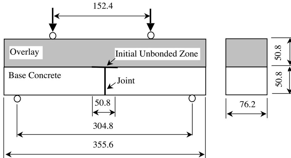
**Figure 2:** Dimension of simulated overlay system and loading configuration.
