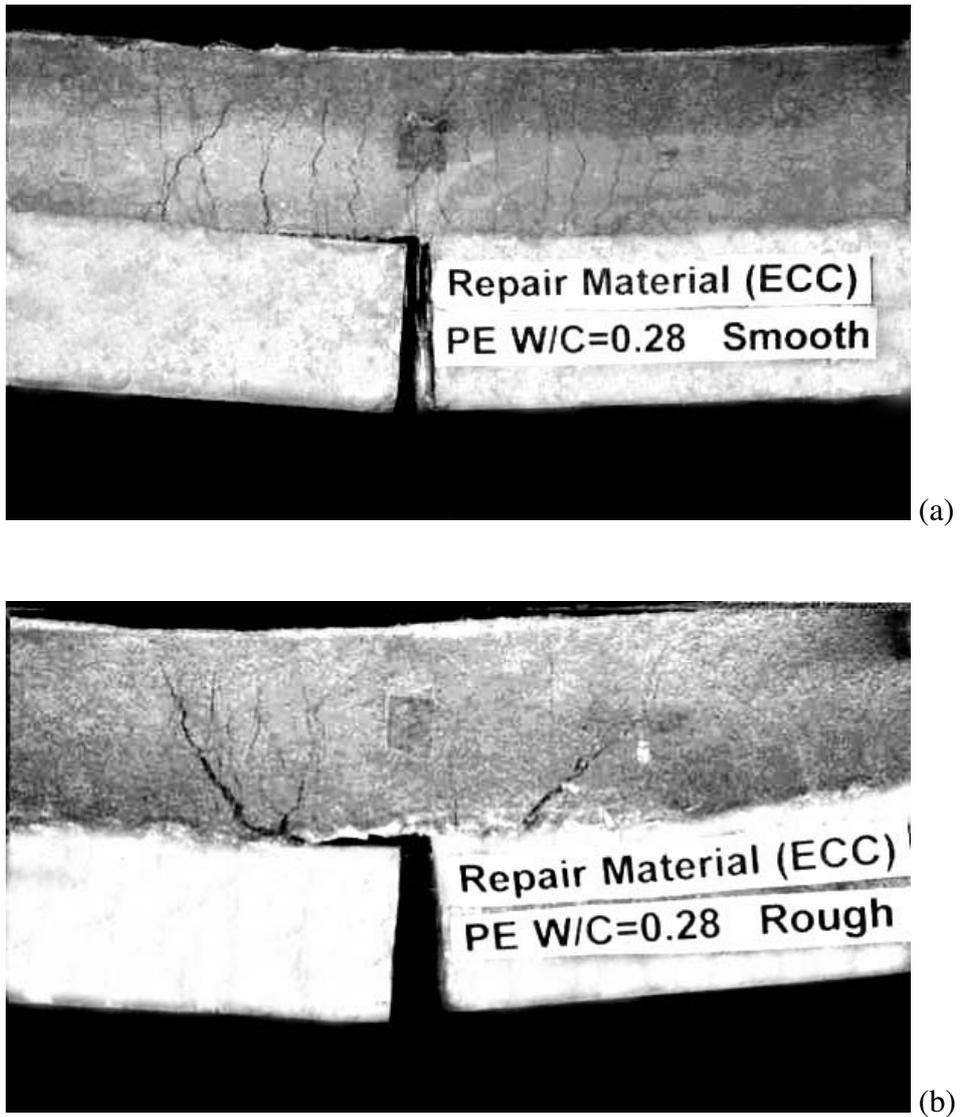
**Figure 7:** (a) The kink-trap mechanism associated with a smooth interface is replaced by (b) a plastic-zone formation when the ECC/PC interface is roughened.
