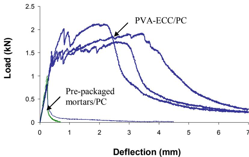
Figure 10: Load-deflection curves of sprayed PVA-ECC/PC overlay systems, showing much higher peak load and deformation capacity in comparison to spray pre-packaged mortars commonly used in concrete structure repair.
