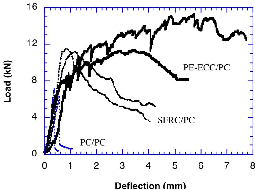
**Figure 5:** Load-deflection curves of the PC/PC, SFRC/PC and the PE-ECC/PC overlay systems.
