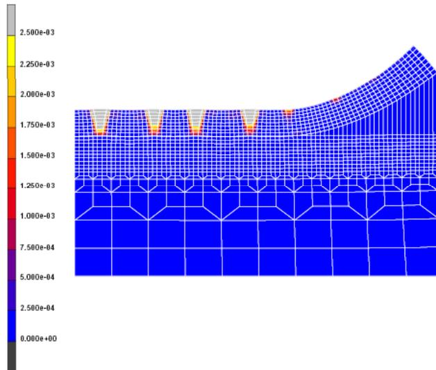
**Figure 13 a):** Contour bands of normal cracking strain (%) on deformed mesh (magnification 100x) for mortar overlay at 16 days
